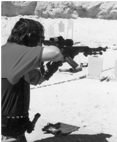
Kelly Beale on the AR-15. Note the double scope on his rifle. Red dot scope for close range, high-magnification scope for long range. (Photo by Robin Taylor.)
